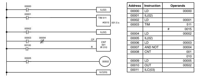
When the execution condition for the first IL(02) is OFF, TIM 511 will be reset to 1.5 s, CNT 001 will not be changed, and 00502 will be turned OFF. When the execution condition for the first IL(02) is ON and the execution condition for the second IL(02) is OFF, TIM 511 will be executed according to the status of 00001, CNT 001 will not be changed, and 00502 will be turned OFF. When the execution conditions for both the IL(02) are ON, the program will execute as written.
